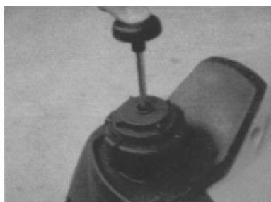
1 – The ventilating pole of fuel-filling lid
