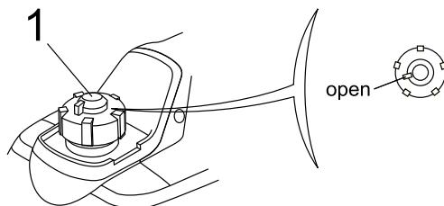
Note: in case of first use or in cold environment fasten the fuel-filling lid till the ventilating pole indicates to OFF
