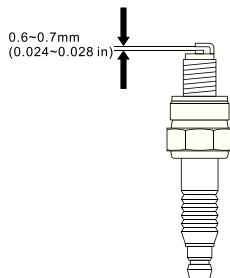
17. Install the spark plug carefully by hand. Pay attention not to overlap the screw thread.
