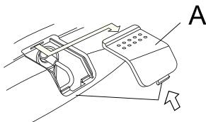
12. Dismantle the cap of the spark plug.
